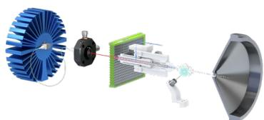
Figure 2 - Schematic of the Luxon ionization source
