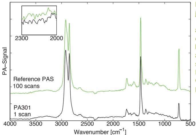
PA301 gives an equal SNR with just one scan, as opposed to 100 scans by its commercial alternative. This means that overnight measurements can be now performed in only a few minutes. A polyethene sample was analyzed with FTIR using resolution of  $8 \text{ cm}^{-1}$ , OPD  $0.16 \text{ cm/s}$ , and using helium purge in both systems.
